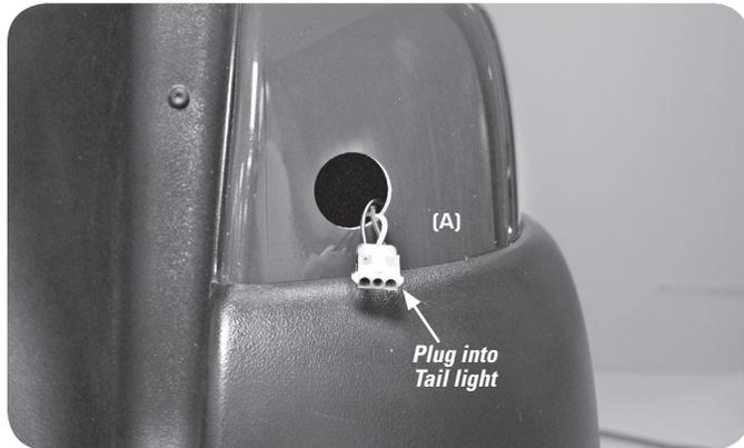
the Tail Light, and position the Tail Light (B) so that it rests on the Bumper and the wide edge aligns with the Bag Well. Secure with Taillight Ring using the provided Hardware (C).
