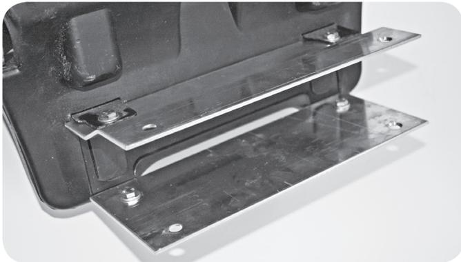
Use the long hardware provided to attach the two Bracket Plates to the Bumper, as pictured below (with stamped "F" facing towards Bumper).
