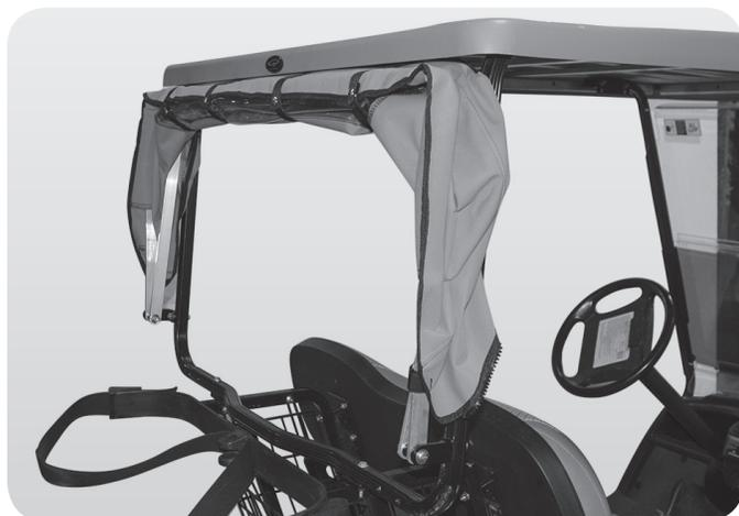
Attach the Bag Cover Brackets to the Rear Frame using the provided hardware (Bolt Head on inside with Nut and Washer outside). (Repeat for other side).
