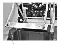
**1)** Lift cargo bed frame & bumper angle assembly off of bumper. Fully tighten bolts connecting the upright supports and the bumper angle.
