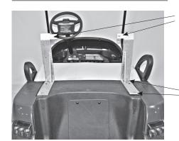
NOTE: The TABs on each seat back support should face to the inside.
