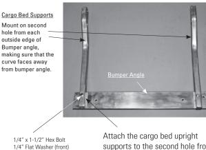
1/4 X 1-1/2 Hex Bolt 1/4" Flat Washer (front) 1/4" Flat Washer (rear) 1/4" Jam Nut (Both Sides)
