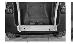
**2)** Lower the cargo bed frame & bumper angle assembly, so that it is resting on bumper again. Make sure Bumper Angle is centered on car bumper. Using one of the two holes in the center of the Bumper Angle as a guide, use a 5/16" drill bit and drill completely thru the bumper. Install mounting hardware. Repeat for other remaining hole.
