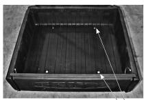
Align the four holes in cargo bed with the four holes in the H-frame. Mount cargo bed using stainless steel hardware on top. 5/16" x 3-1/4" SS HEX Bolt 1" SS Washer (top) 5/16" Flat Washer (bottom) 5/16" Nyloc Nut (bottom) (2x Both Sides)
