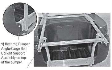
1/4" x 2-1/2" HEX Bolt 1/4" Flat Washer (front) 1/4" Flat Washer (back) 1/4" Nyloc Nut (Both Sides)
