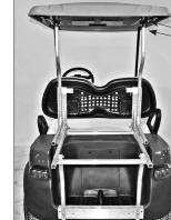
Use the factory hardware to mount factory top to front frame and to rain cups on 84PRE Strut Kit. **FULLY TIGHTEN**
