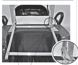
Cargo Bed H-frame Base NOTE: Attach the H-frame to seat back supports. Use the end of H-frame that extends furthest past the cross bars and has a hole located 1/2 inch from end.
