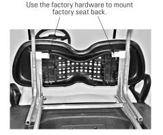
Mount the factory seat back to the seat back supports, using original factory hardare.
