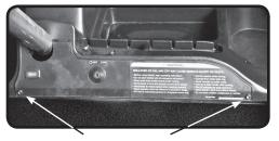
Remove the Ingnition Switch Panel by removing the Torx head screws.
