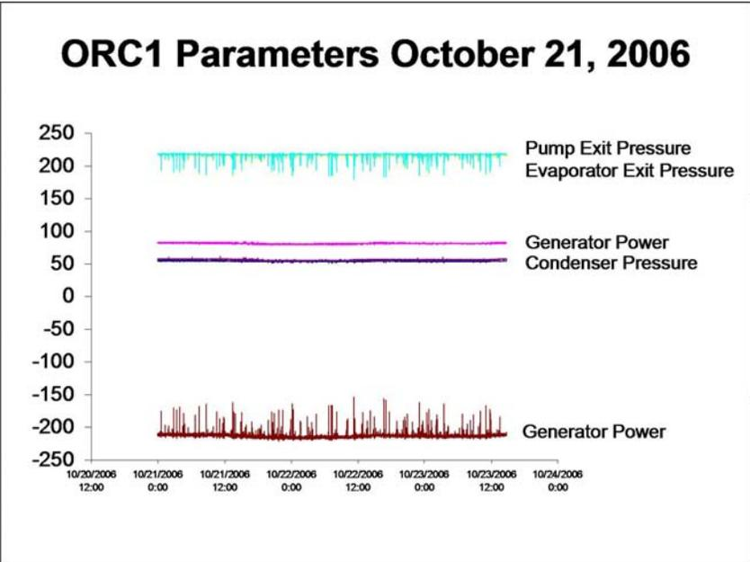
**Figure 4:** Sample of data collection and tracking of limited number of parameters from ORC1 from October, 2006.
