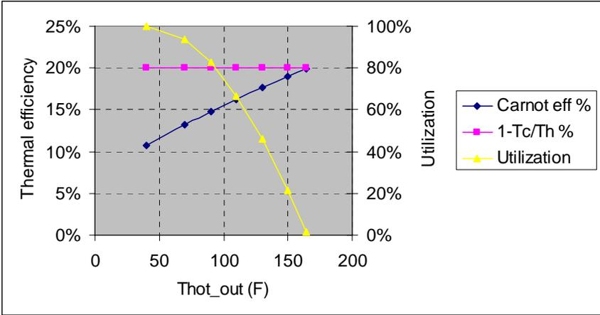
**Figure 3:** Carnot efficiency and utilization for limited hot resource. ( $T_{hot\_int} = 165\text{ }^{\circ}\text{F}$ ,  $T_{cold} = 40\text{ }^{\circ}\text{F}$ )
