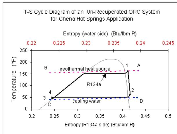
Figure 7. Temperature-entropy diagram of the proposed Chena Hot Springs ORC unit
