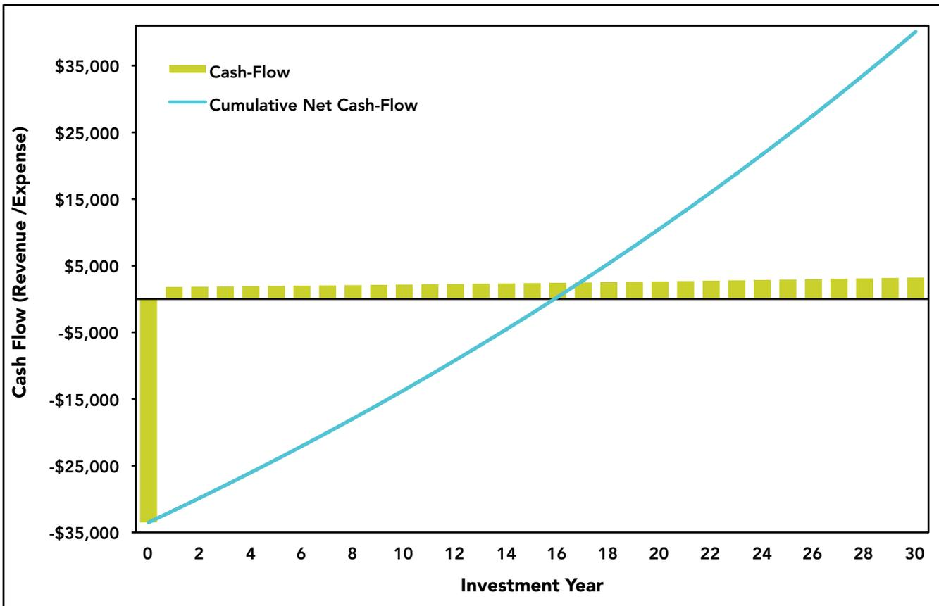
Figure 6: Example 30-year nominal dollar cash flow for a well-sited, well-maintained small wind turbine
