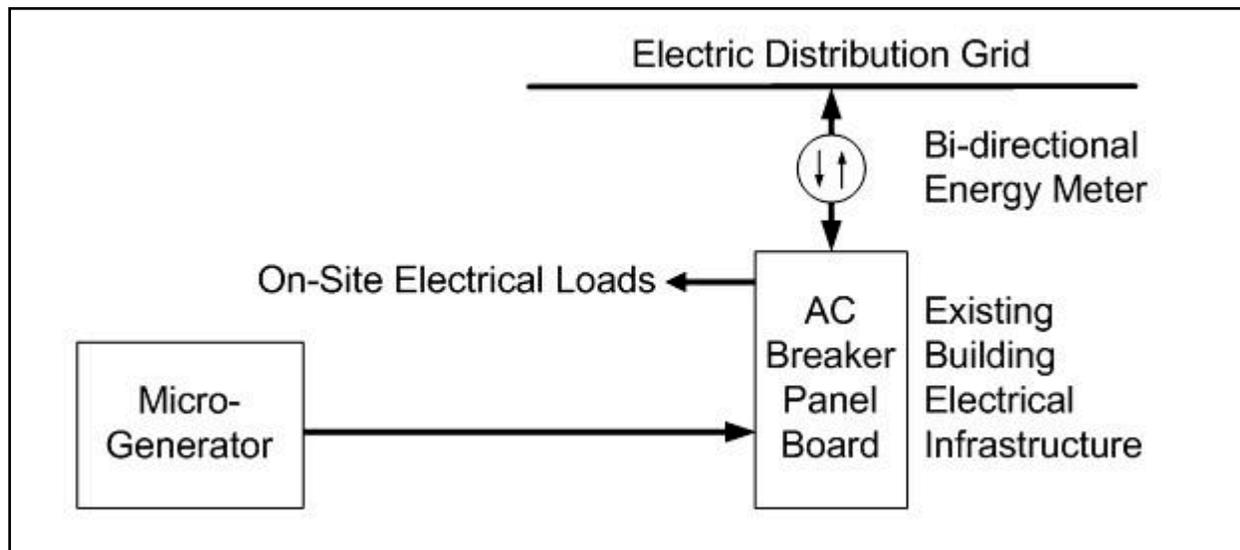
Figure 20: Typical configuration of a micro-generator to grid connection
