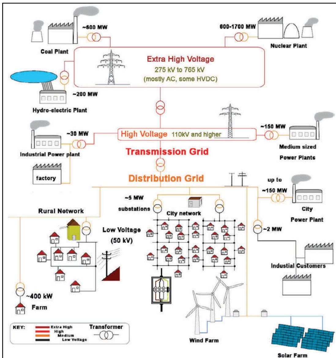
Figure 7: Example of typical components of the electric grid
