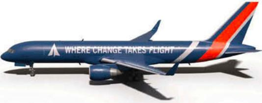
Weighing in with an OEW as low as 115,500 lb., the Precision conversion is the lightest 757 conversion in production today. With the highest available payload of any converted 757, plus winglet compatibility, Precision Aircraft Solutions is the undisputed conversion champion.
