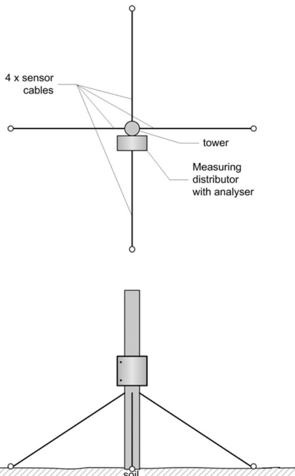
Fig. 9: Slope set up SWS with 4 sensor cables
