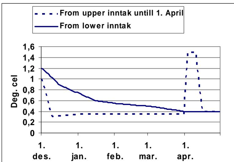
Figure 4. Temperature measured in the water from the power station when using the lower intake (up to 2002) and when using the upper intake (after 2002).
