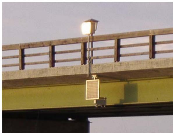
Figure 18. Solar powered RQ-24 and radio transmission.
