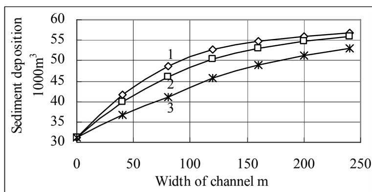
Figure 2. Dependence of average amount of sediments settled during one year on width of channel, when depth of channel is: 1 – 3.0 m, 2 – 2.5 m, 3 – 2.0 m.
