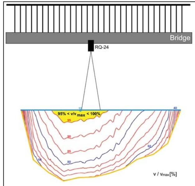
Figure 2. Measure the local velocity  $v_l$  at the radar measurement spot. The factor  $k$  converts the local velocity  $v_l$  to the mean velocity  $v_m$ .
