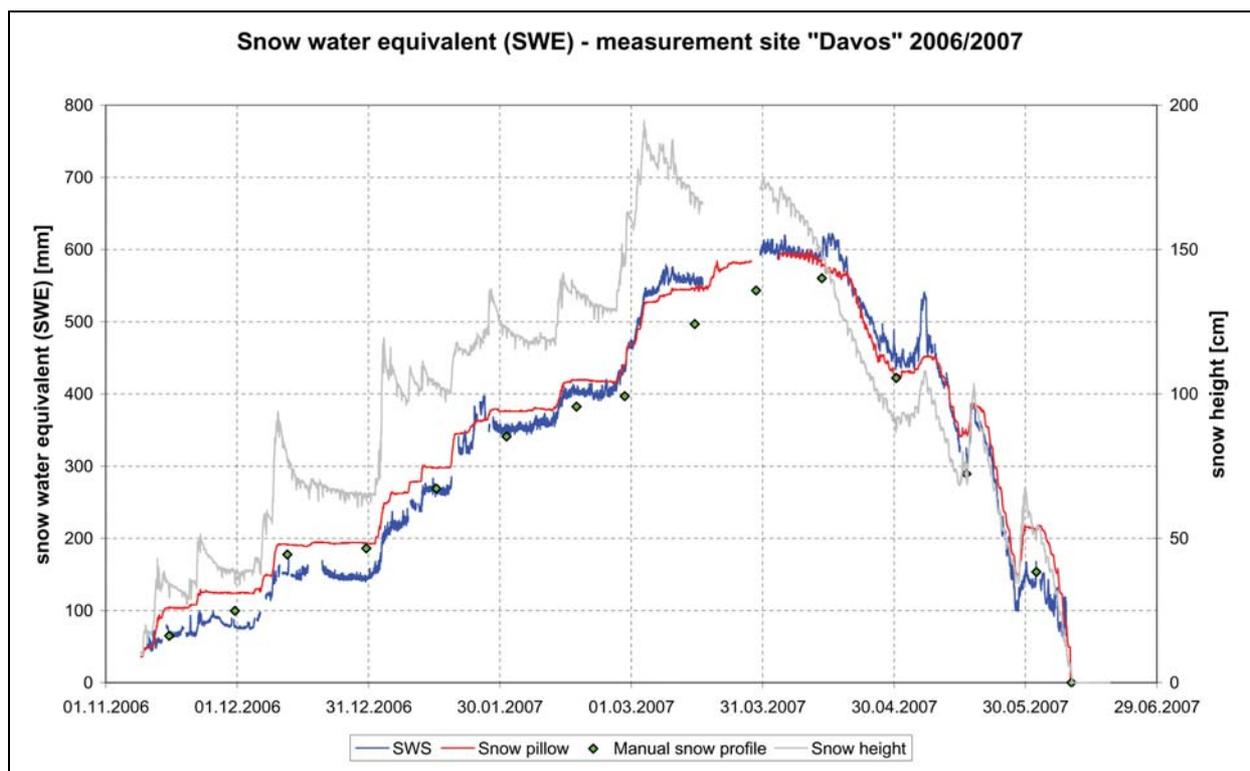
**Fig. 5: Measurement of snow water equivalent (SWE) by the snow water sensor (SWS) compared to different measurement methods.**
