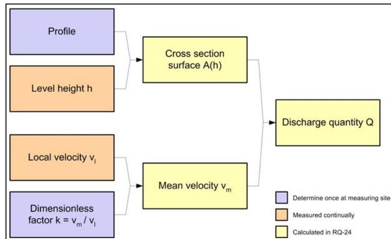
Figure 1. Measuring principle of RQ-24 system.
