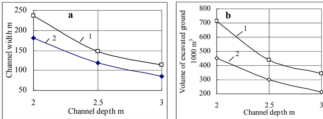
Figure 3. The necessary channel width (graphs a) and the ground volumes, necessary to excavate from the channel, (graphs b) dependences on the channel depth, when the desirable increase of sediment deposition in the valley after arrangement of channel is: 1 – 70% 2 – 50%.
