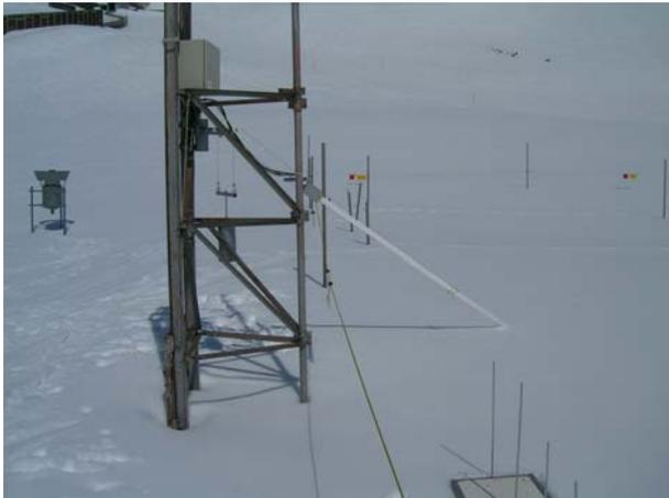
Fig. 1: White sensor cable mounted at tower with analyser unit (grey cabinet)
