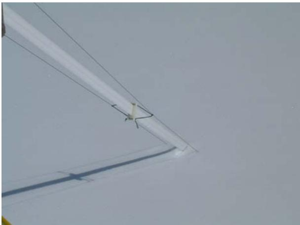
Fig. 3: White sensor cable with guidance cable and integrated temperature sensors
