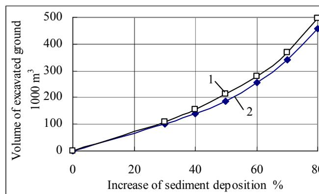
Figure 4. Dependence of ground excavated from 1 meter of channel length on the desirable increase of sediment deposition in the valley: 1 – when channel depth is 2.5 m; 2 – when channel depth is 3.0 m
