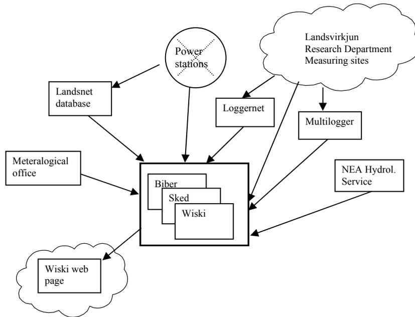
Figure 1. The integrated measurement system of Landsvirkjun.
