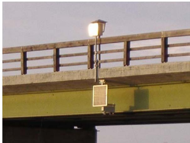
Figure 18. Solar powered RQ-24 and radio transmission.
