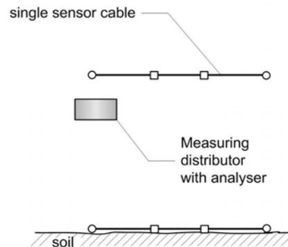
Fig. 11: Horizontal set up SWS single sensor cable
