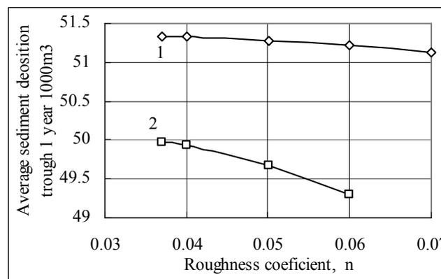
Figure 6. Influence of the reserve road dyke existence and growing of bush or wood strips in the valley on sediment deposition in the valley, when: 1 – the reserve road dyke is absent; 2 – the dyke exists.
