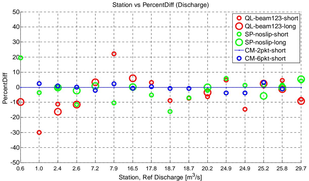
The table below shows mean and median values for discharge. We observe that compared to current meter 2 points per vertical, current meter 6 points performs best. It is followed by StreamPro as second best, and then by QLiner. For StreamPro and QLiner those with long averaging interval perform better than those with short averaging intervals. Observe that all instruments measure smaller discharges than the 2 points current meter measurements.
