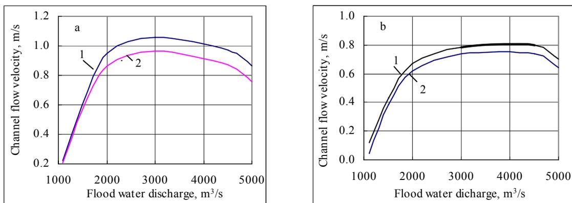
Figure 5. Water velocities developing in the channel, when its depth is: a – 3 m; b – 2.5 m and when the width of channel is: 1 – 100 m, 2 – 160 m.
