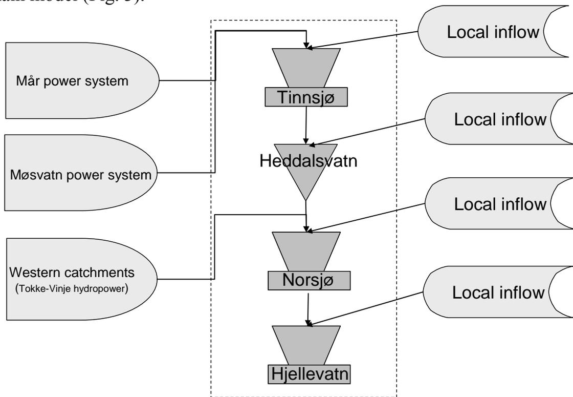
Figure 3. Components in the flood warning system.
