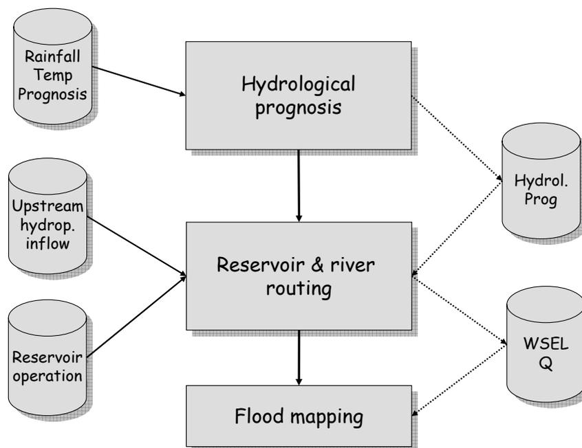
*Figure 1. Structure of the Telemark floor warning system. The storage on the left hand side symbolizes external input data to the system, and the right hand side shows the internal data flow.*
