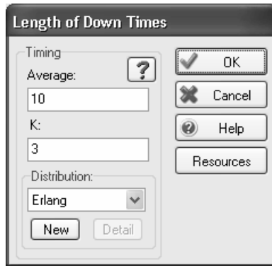
Figure 9-11 The length of time that a work center is down during a breakdown can depend on resource availability.
