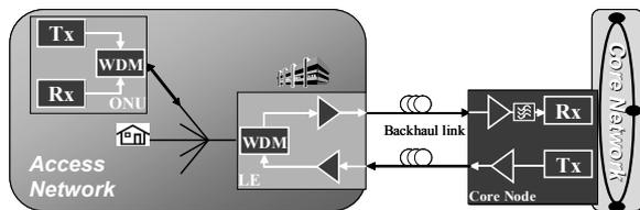
Fig. 1: Architecture of long reach amplified PON.
