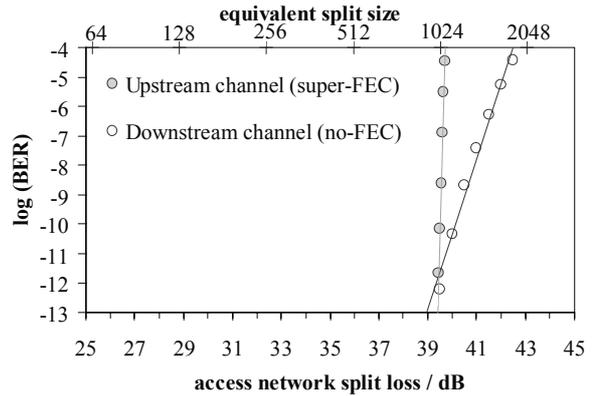
Fig. 7: BER vs. access network loss, for both upstream and downstream channels in LR-PON.
