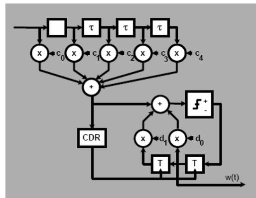
Fig. 5: Block diagram of electronic dispersion compensation chip.
