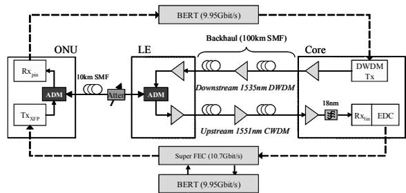
Fig. 4: Layout of LR-PON system experiment
