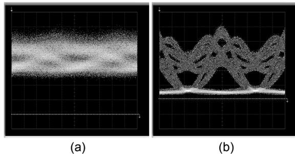
Fig. 8: Eye diagrams of: (a) of upstream signal recorded at OLT Rx input and (b) downstream signal recorded at LE output. (Horizontal white line indicates zero level.)
