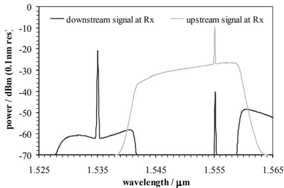
Fig. 9: Spectra recorded at receiver inputs for both upstream and downstream channels in LR-PON.
