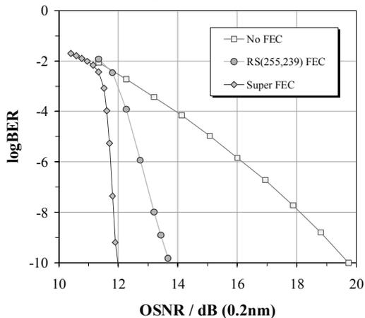
Fig. 6: BER vs. OSNR for various FEC configurations as measured over upstream LR-PON path.
