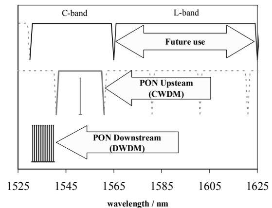
Fig. 2: Example wavelength plan for LR-PON.
