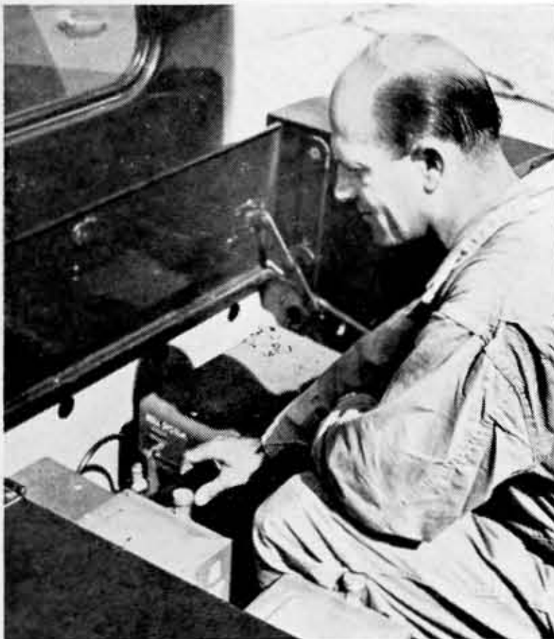
THE SET is a compact radio unit housed in a box behind the cab. The signal is picked up by transmitters and carried through normal telephone channels.
