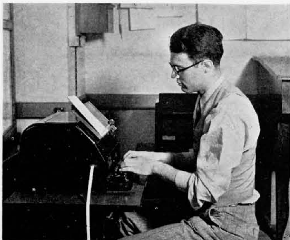
Teletypewriter on which weather reports for the guidance of aviation are sent and received.
