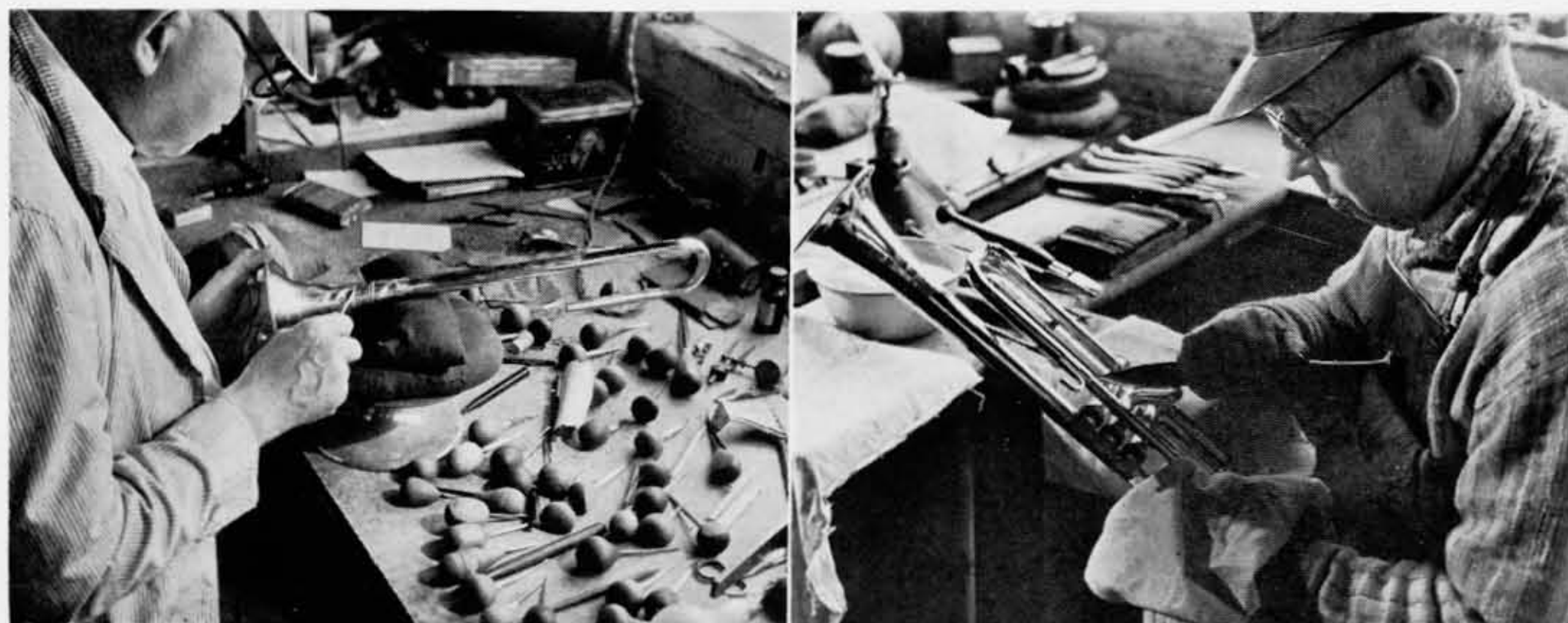
Left—The engraver putting a design on the "bell" of a nearly completed cornet. Right—The burnisher's job is a slow one. Note how small is the point of his burnishing tool.
