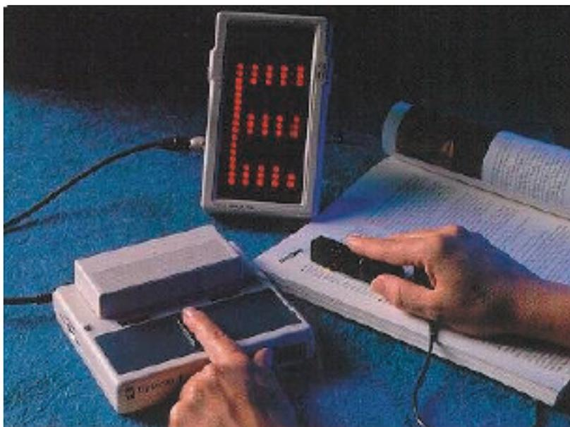
Figure 2: Optacon incorporates OCR with tactile Braille feedback
