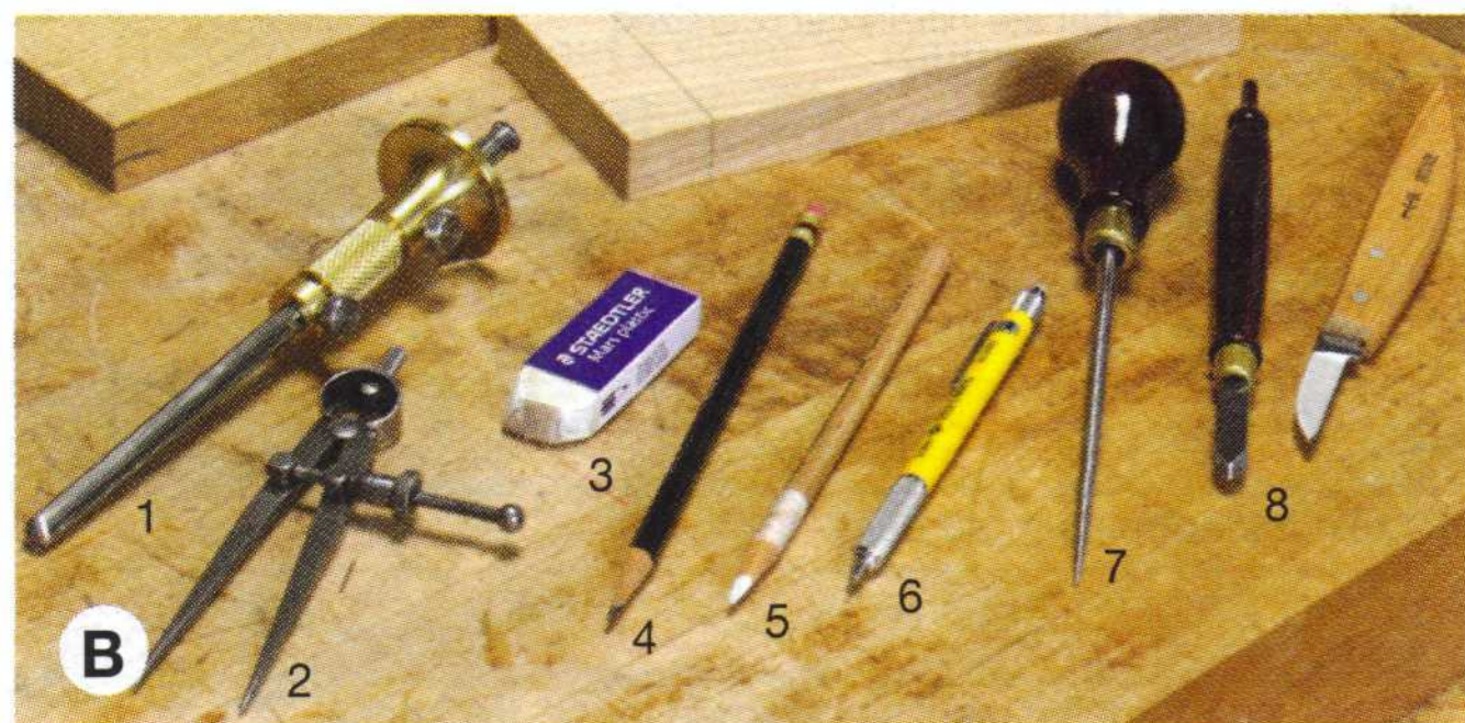
Keep this marking tool set near your bench. Pencil lines are easier to see, but scribed lines cut more cleanly.
