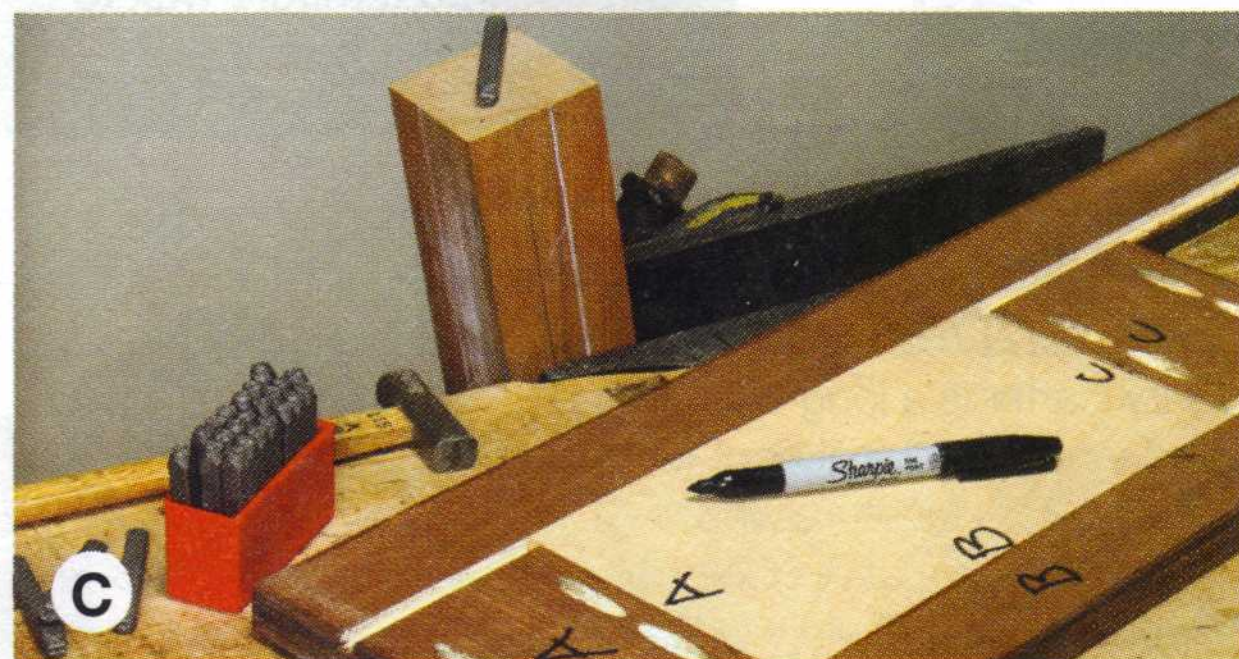
Use a marking pen or stamped letters to mark parts in order to avoid confusion during assembly.
