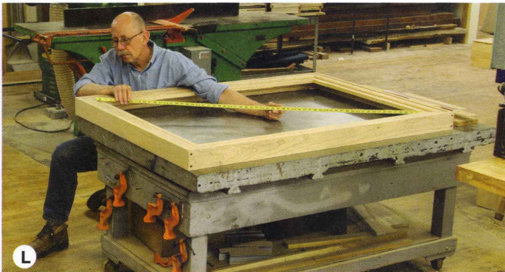
Large frames deserve square corners. Use a folding rule to measure the diagonals. When the dimensions are equal, your frame is square.
