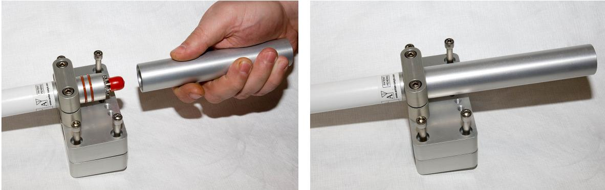
The mast mount can accommodate a wide range of mast sizes from approximately 1 to 3 inches. The antenna clamps can also be used to attach the antenna to other flat surfaces. The hole spacing of the symmetric antenna clamps is 1.5-in. (38.1mm). The antenna base accommodates through-bulkhead applications; contact the factory for custom solutions.
