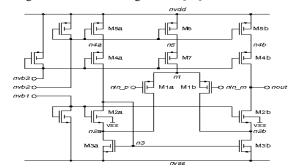
Figure 5: A CMOS Operational Transconductance Amplifier, used to generate datasets for six SR problems
