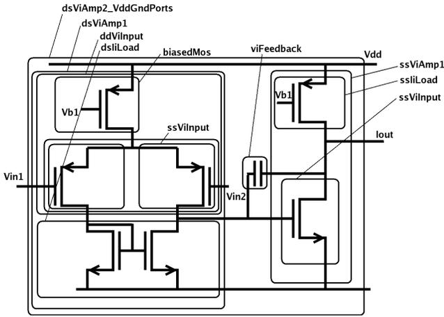
Fig. 7. An example individual (“PMOS-input Miller OTA”) shown in schematic form, annotated with MOJITO building block labels.
