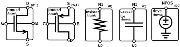
Fig. 3. Example atomic blocks: nmos4 transistor, pmos4 transistor, resistor, capacitor. Example of ports and input parameters: nmos4 has four external ports: *G*, *D*, *S*, and *B*; it has two input parameters, *W* and *L*. Note how *dcvs* (DC-controlled voltage source) has only one external port; the other port ties directly to ground.
