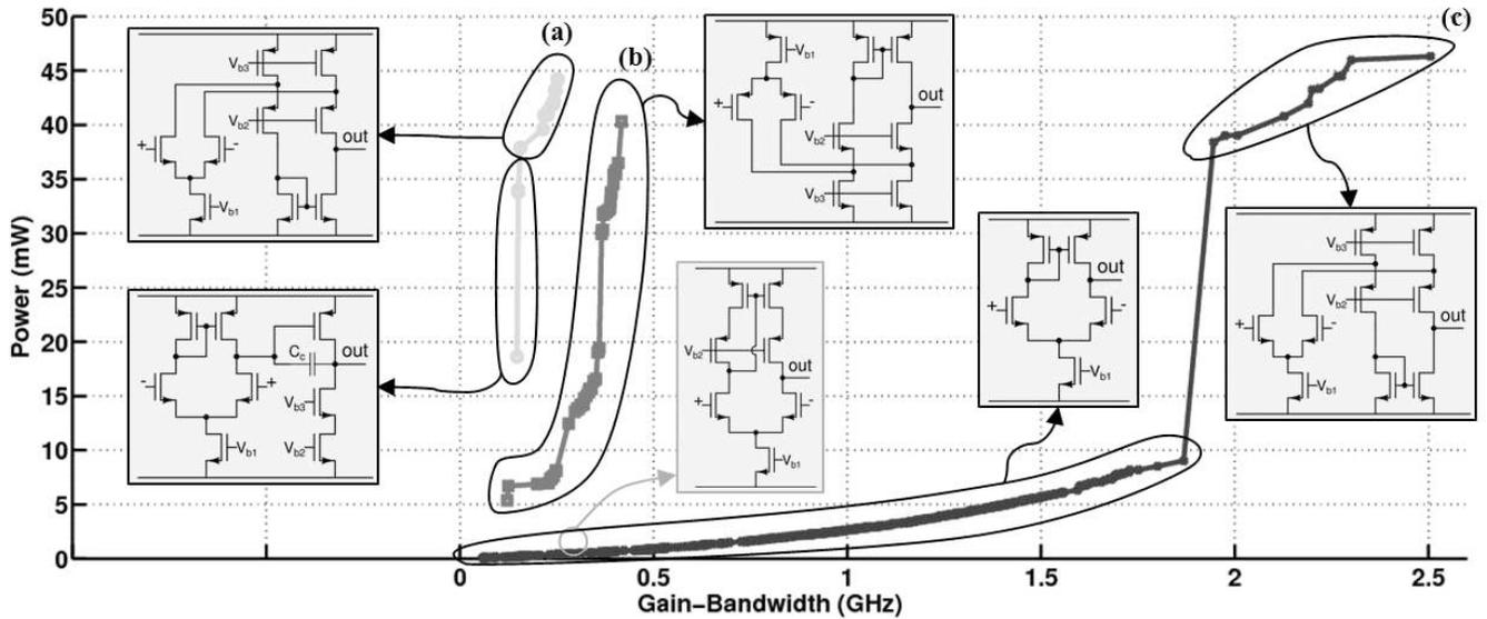
Fig. 9. Combined result plot for 3 synthesis runs. Set (a) shows a Pareto front for  $V_{cmm,in} = 1.5$  V, set (b) is for  $V_{cmm,in} = 0.3$  V and set (c) is for  $V_{cmm,in} = 0.9$  V. Aim is to minimize power and maximize Gain-Bandwidth. Each point is a sized topology; each topology has many different sets of sizings. The expected topologies were found.
