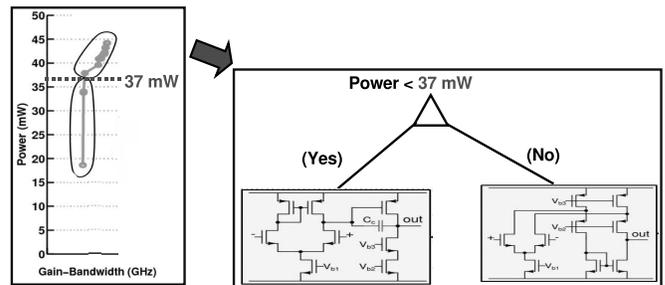
Fig. 14. Left: results of a two-objective run (minimize power, maximize Gain-Bandwidth  $GBW$ ) which gave two topology choices indicated by the ellipses. Right: corresponding a decision tree to guide the topology choice based on the power input specifications
