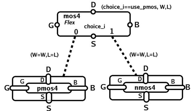
Fig. 5. Example flexible block: *mos4* turns the choice of NMOS vs. PMOS into a parameter "chosen\_part\_index". Note how parameters get assigned from *mos4* to either of its sub-blocks. In this case both sub-blocks use the *mos4*'s *W* and *L* parameters as their own *W* and *L* values.
