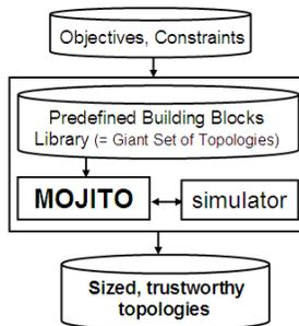
Fig. 2. Proposed flow using MOJITO-R for trustworthy-by-construction analog topology synthesis. A small library of analog structural building blocks combine hierarchically to create a *massive* library of possible topologies. MOJITO outputs sized topologies which are Pareto-optimal according to the objectives of area, power, performances, and *yield*.
