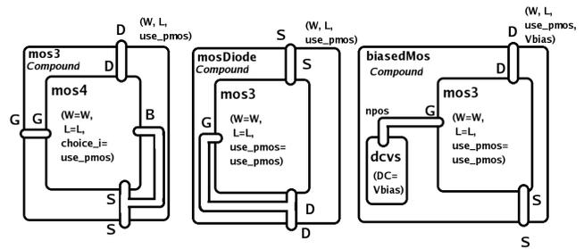
Fig. 4. Example compound blocks. *mos3* is a wrapper for *mos4*, so that the *mos4*'s 'B' node is not seen at higher levels. *mosDiode* ties together two internal ports to only present two external ports. *biasedMos* uses a 1-port *dcvs* (dc-controlled voltage source) block to set its gate bias internally.
