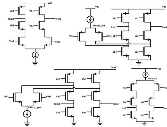
Fig. 6. Four circuits with similar conceptual behavior, but dramatically different phenotypes. The circuits on the left have PMOS inputs, and on the right have NMOS inputs (*input\_is\_Pmos* = True/False). The load's rail is *vdd* in the top row, and *gnd* in the bottom row (*loadrail\_is\_vdd* = True/False).
