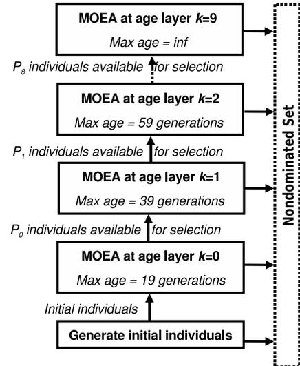
Fig. 8. Structure of MojitoSynthesis(), which uses an age-layered population structure (ALPS) and adds multi-objective support via multi-objective EA selection at each age layer.
