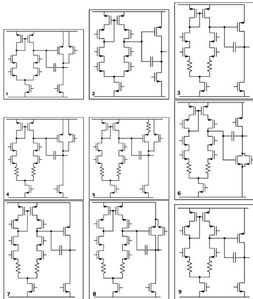
Fig. 12. Topologies in the MOJITO-R experimental run’s Pareto front. A hanging gate implies either a bias voltage source connection or input node. Parallel connected transistor pairs are combinations of a second stage amplifier transistor and a biased transistor (a constant current source).
