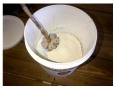
4. Mix briskly with a paint mixer that is similar to the one in picture at the bottom of this page
