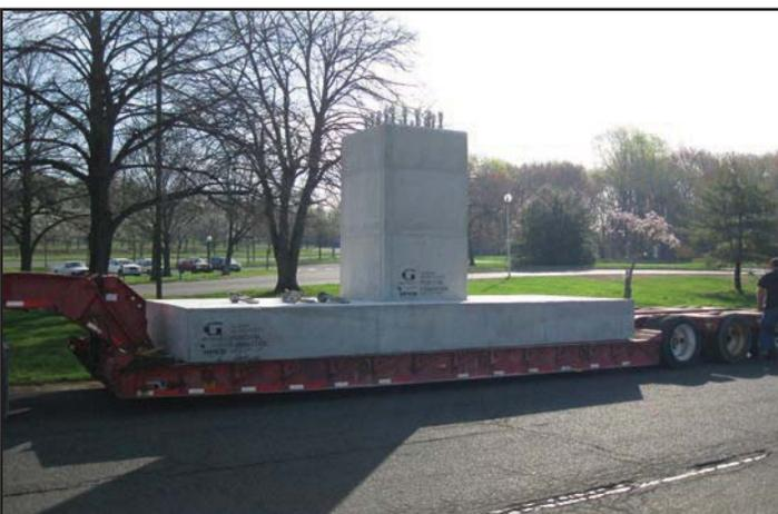
**A pedestal foundation structure is transported to a project.**
