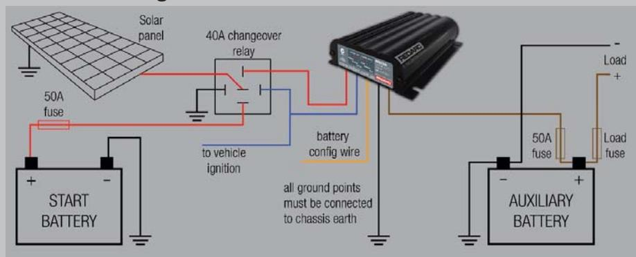
The battery type is set by connecting the orange wire to either ground, positive supply or left unconnected during installation. The BCDC1240 will check the status of this wire on power up and display the selected battery type via the LEDs on the unit.
