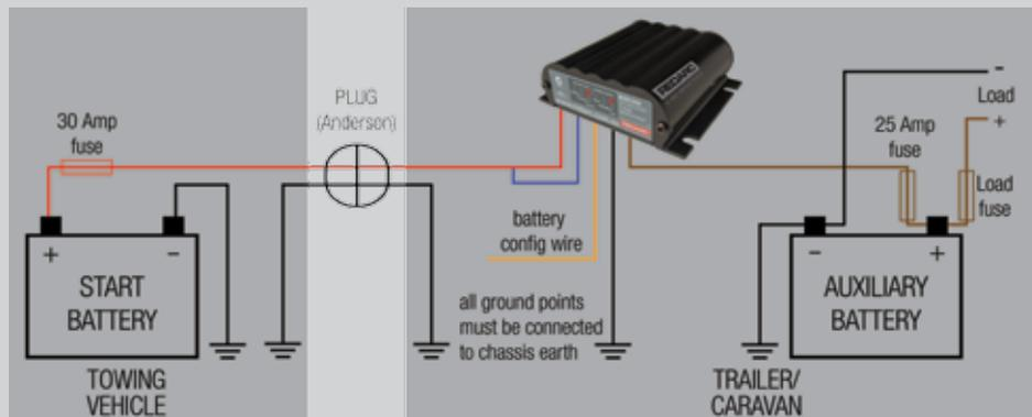
The battery type is set by connecting the orange wire to either ground, positive supply or left unconnected during installation. The BCDC1220 will check the status of this wire on power up and display the selected battery type via the LEDs on the front of the unit.
