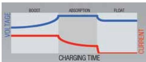
Simply select the battery type at installation to ensure your battery receives the optimal charging profile specific to that battery's chemistry.
