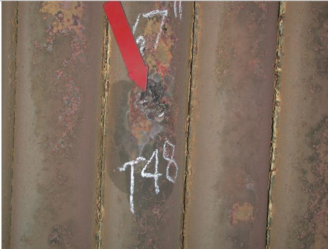
**We often use visual inspection to select areas that would require further examination by an NDT method. In this case deposits on furnace waterwalls were selected for more detailed examination by Magnetic Particle.**
