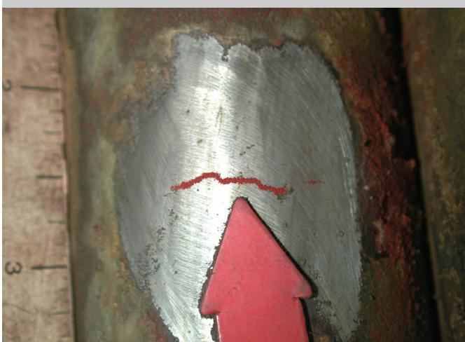
**Magnetic Particle revealed cracks that were attributed to overheating of the tubes from heavy scale deposits. The knowledge gained by experience in Boiler and Pressure Vessel Inspection aids in the choice the test area.**
