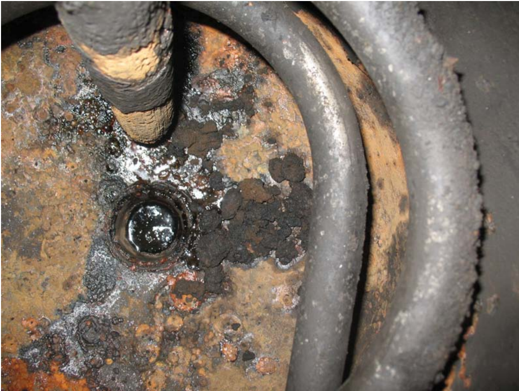
Internal Corrosion observed remotely inside a pressure vessel & verified with external B-Scan UT.
