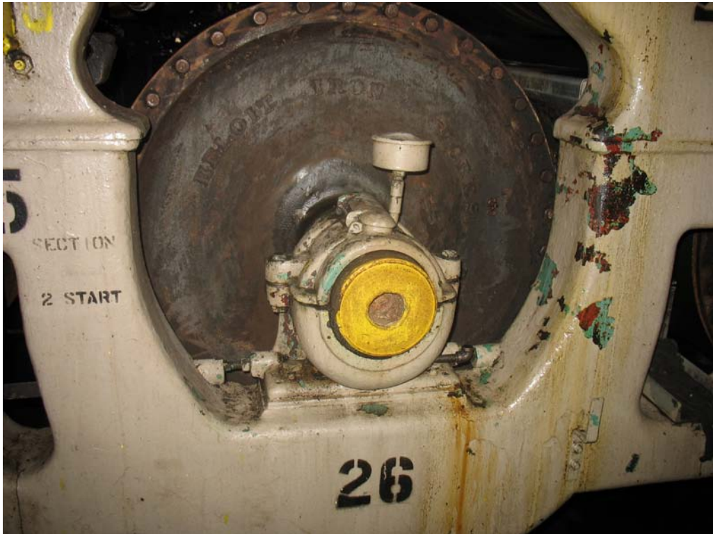
The journal area of each dryer is checked for cracking that could lead to a failure.
