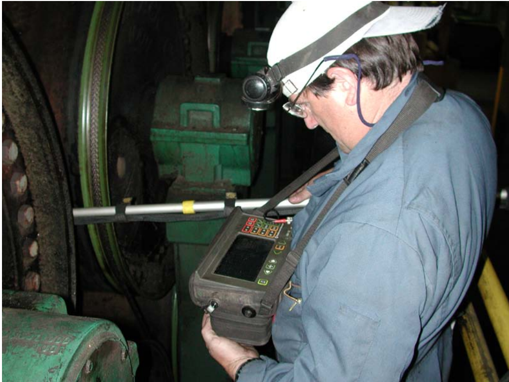
Technician controls the progress of the scan manually across face.
