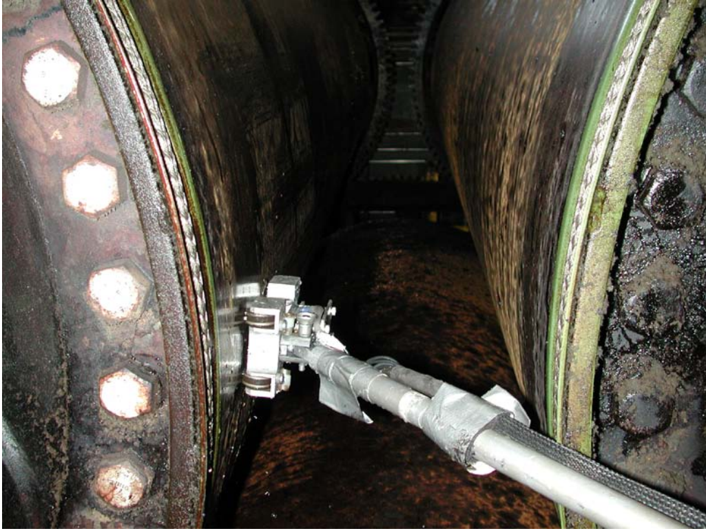
Four magnetic wheels hold the transducer cart on the roll. The clearance is about 4"-5" in a vertical direction to allow the cart to travel along the roll.
