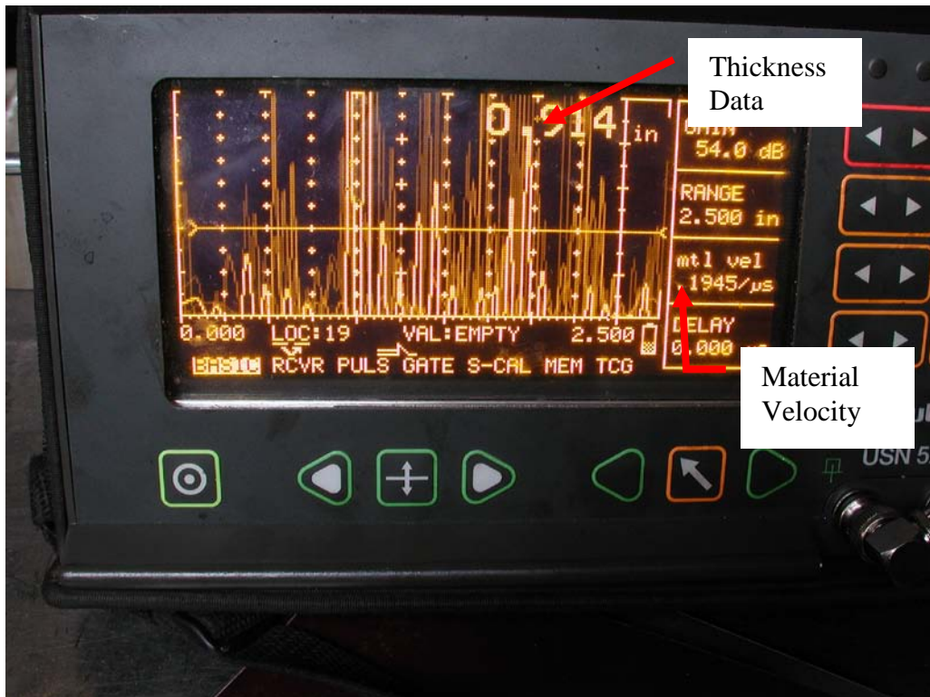
The system can read both the dryer wall thickness and the material velocity.
