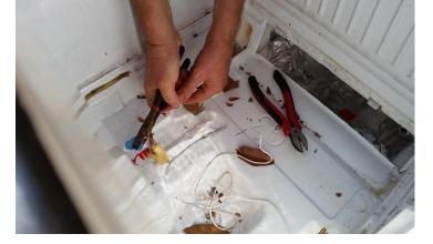
including shelving. Plug any holes in the bottom or back of the fridge to prevent water leakage, using silicon sealant.
