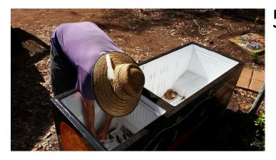
5. Ensure water can pass through from the main reservoir to the freezer area. If not, drill a hole through low down, using a 25mL holesaw drill bit.
