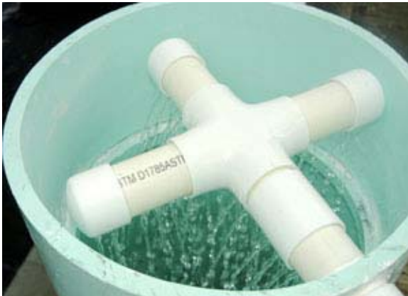
Top of tower with out drip plate to show fabrication of shower head and water distribution
