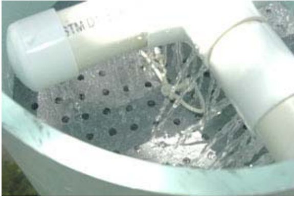
Close up of top of tower with drip plate
