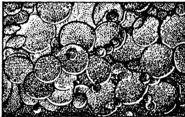
Figur 8 Frazil ice has the form of small platelets 4-8 mm in diameter and 0.1 mm thick.
