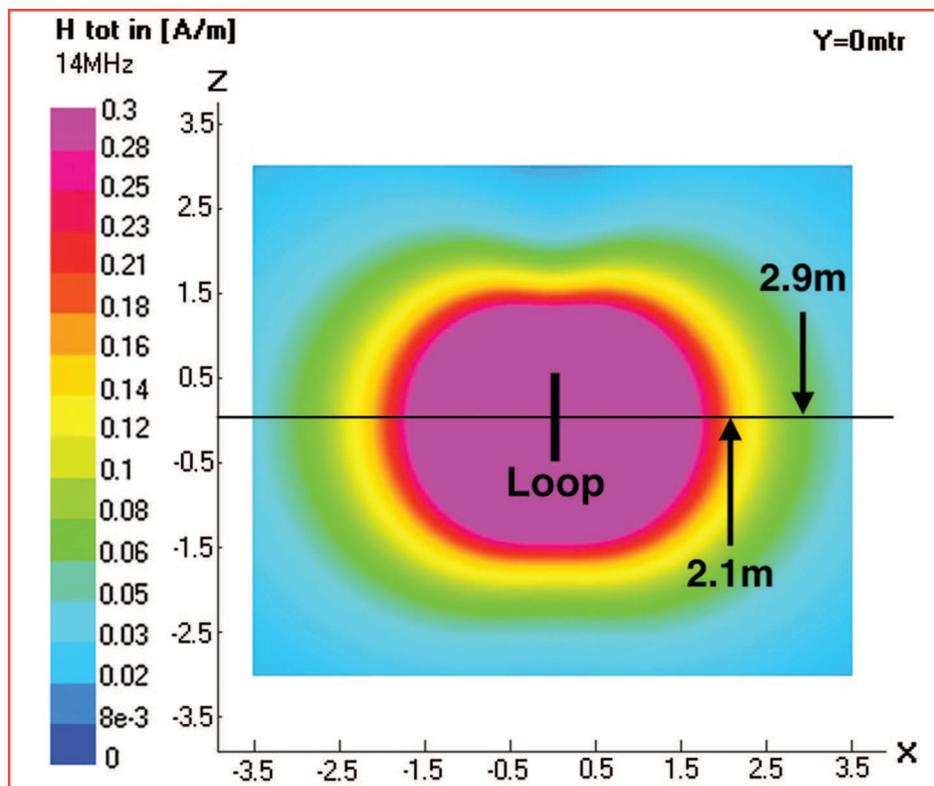
**FIGURE 1:** Contour plot of magnetic induction H for 10 watts at 14MHz. Occupational and public safety distances are indicated on the perpendicular axis of the loop.
