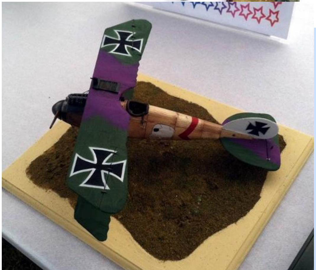
Part of the IPMS Display 1/32 SCRATCHBUILT Albatross. Each panel is separately made and the wings are fabric
