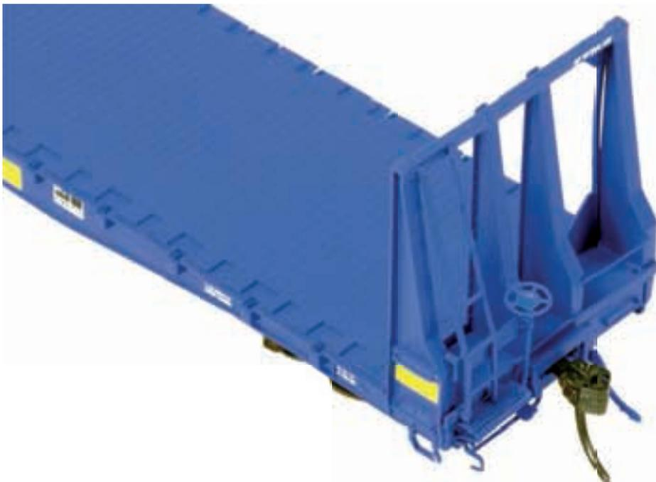
this model, he observed these panels in various stages of disintegration on frequent examples. To allow the hobbyist freedom to conjure up these panels in realistic-looking rough condition, the model release went with providing pristine panels separately to keep options on this area open.
