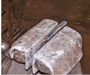
Figure 9 Vise as a heat sink
