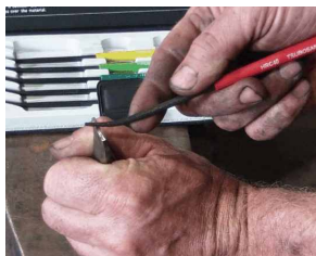
Figure 12 The 40 HRC file slid over the metal
