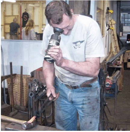
Figure 3 A pyrometer is used to insure that a heat of 830 to 880 degrees is reached
