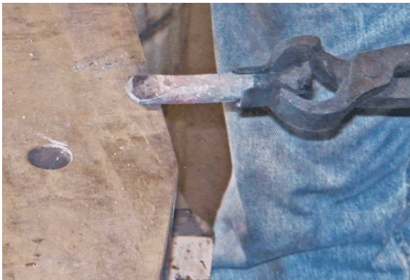
Figure 1 Forging the cutting end
