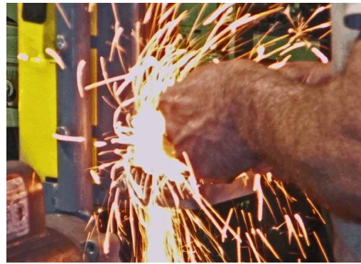
Figure 4 Grinding the cutting edge
