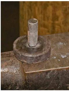
**Figure 9** Stub in tool
