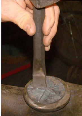
**Figure 14** Creating chisel lines
