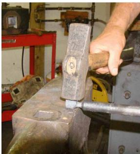
**Figure 4** Shouldering on anvil
