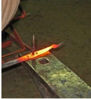
Step seven: Use half face strikes to start a tail, make sure the tail is going in the opposite direction of the beak.
