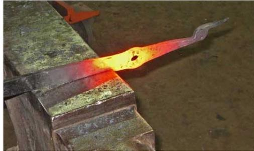
Step eight: Transfer the swan to the vise to clean up the tail with chisel.
