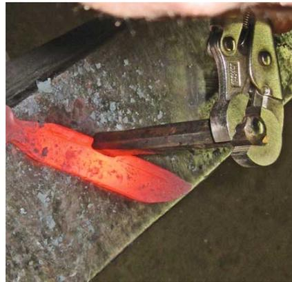
Step thirteen: Use a teardrop tool to create the feathers. Remember you need two wings and you need to texture them, create the feathers, on opposite sides. Cut the wing off, punch a hole for the rivet, clean up the round and assemble and rivet the wings to the body.
