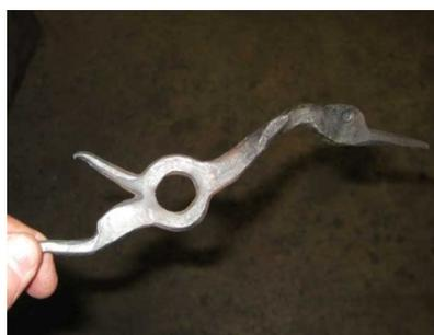
Step one: Using the near side of the anvil and half face blows you create a step and isolate the material for the beak.
