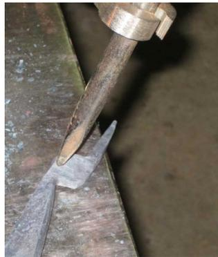
Step five: Slot punch for the rivet to hold the wings. A punch is used to add volume to the body. Drilling a hole would simply remove stock.
