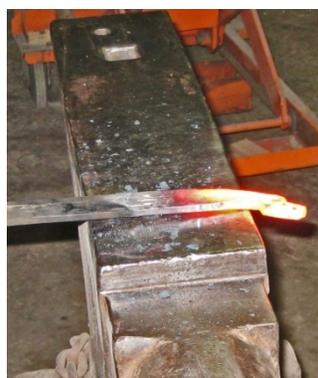
Step three: Round out the edges and draw out the beak.
