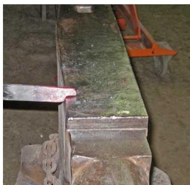
Step two: Using the far side of the anvil and half face blows you isolate the material for the head.
