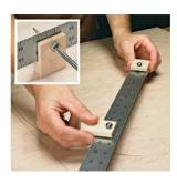
Received this jig suggestion via email: In the past, when I had to lay out a large circle or arc, I usually resorted to making a compass specifically for that application. Recently, however, when faced with the prospect of making yet another single-use compass, I decided to build this
