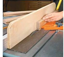
That led me to build an L-shaped accessory that attaches to the rip fence on the table saw (see Photo above). It creates a "zero-clearance" opening that provides support for the workpiece right up next to the dado blade. As a result, there's no way for the piece to drop into the opening. And since the wood fibers are fully supported, tearout is virtually eliminated, which improves the quality of cut.
