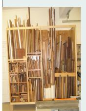
designed to allow ease of access, good visibility of contents, and accommodation of a wide range of wood dimensions including a rear pocket for sheet goods. *Fine Woodworking* published an article on this rack in the *Methods of Work* section of their Dec, 2013 issue. This will be a PowerPoint presentation with photos of the construction details, dimensions, features, and subsequent modifications.
