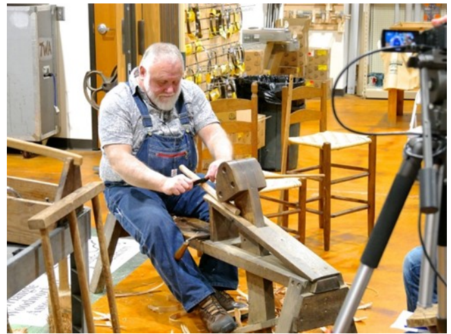
Shaping the legs using a riving knife and shaving horse (photo: Mark Firley)
