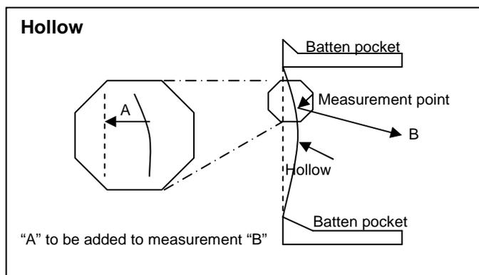
8. Add any **hollow (A)** to each measured **Width (B)** to get the final **widths**.
