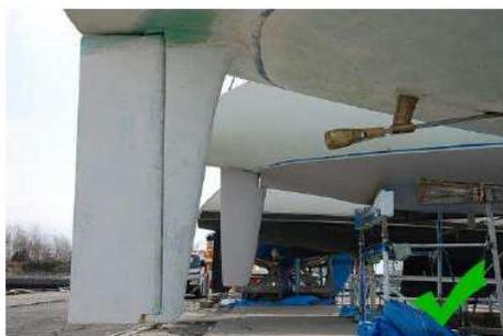
Skeg clearly visible as is propeller
