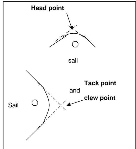
6. Fold the **head point** to the **tack point**. Mark the fold. That is **half luff point**.
