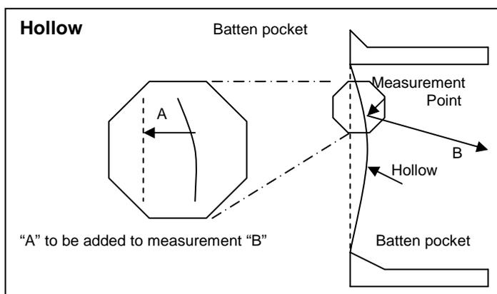
10. Add any **hollow (A)** to each measured **width (B)** to get the final **widths**.
