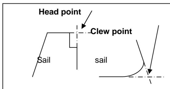
4. Fold the **head point** to the **half leech point**. Mark the fold. That is **three quarter leech point**.
