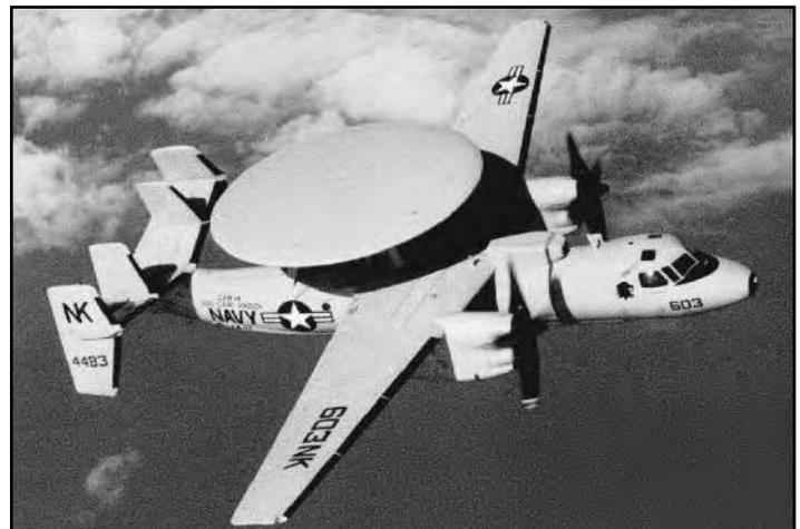
E-2C Hawkeye – Navy's all-weather, carrier-based tactical battle management airborne early warning, command and control aircraft for the Carrier Strike Group and Joint Force Commander.
