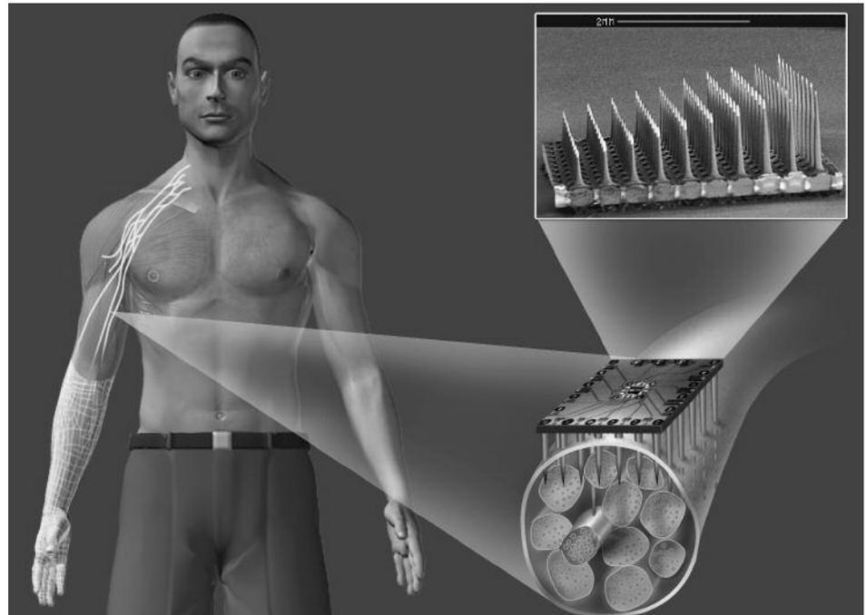
Figure 6: *The Use of the Utah Slanted Electrode Array in the Measurement of Peripheral Nerve Activity*<sup>9</sup>
