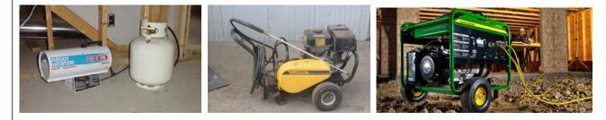
CO results from the incomplete combustion of materials containing carbon (fuels), anything that will burn. It has about the same specific gravity as air, so it can disperse easily throughout the workplace. Pockets can form in areas with little air movement.
