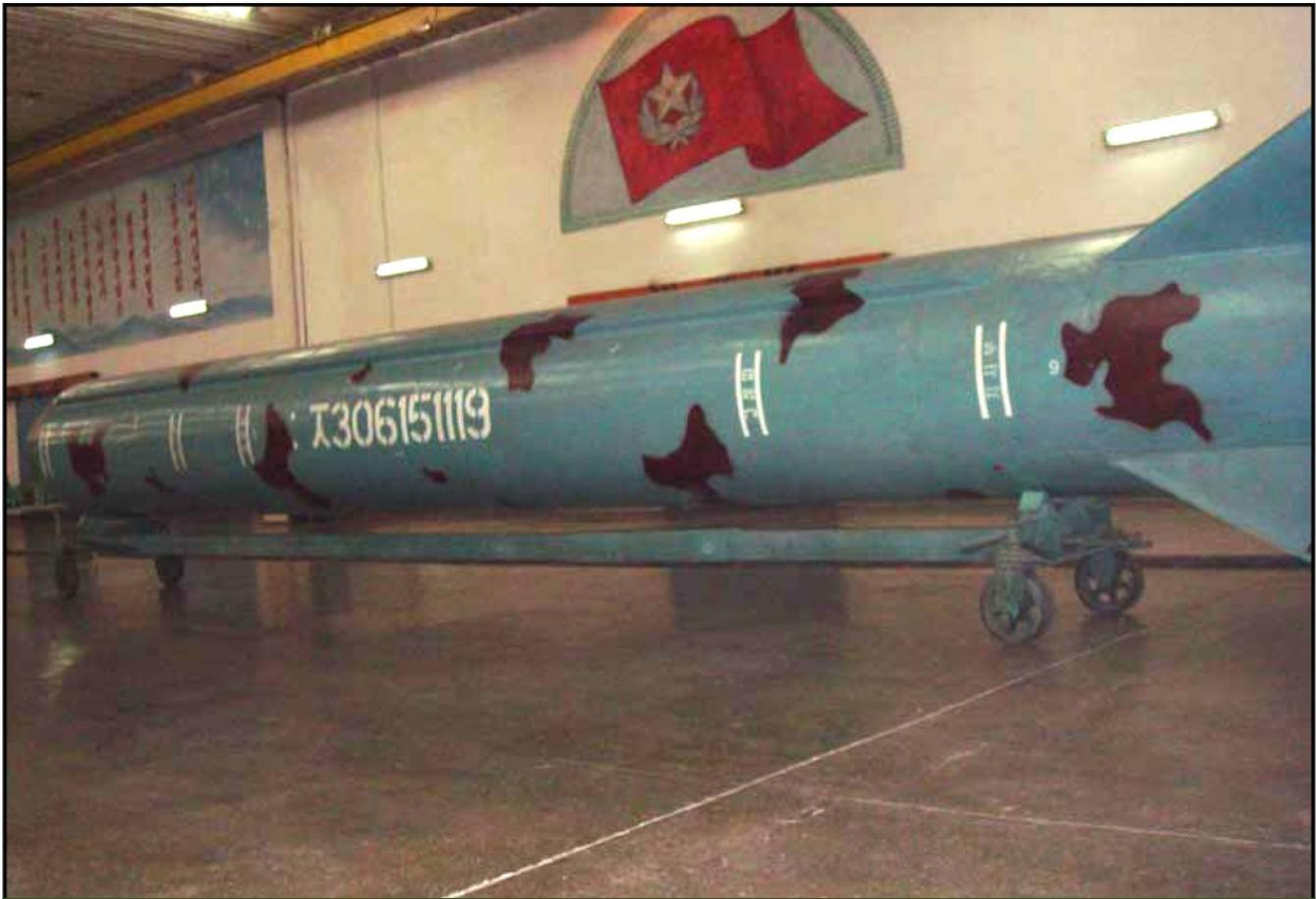
An image of a Nodong on its construction trolley taken by the Myanmar military delegation during its November 28, 2008 visit to the Tae-sung Machine Factory. Early in the ballistic missile program the numbers painted on the missile's airframe had meaning, however, today they are there for display or deception purposes only, as is the camouflage scheme.
