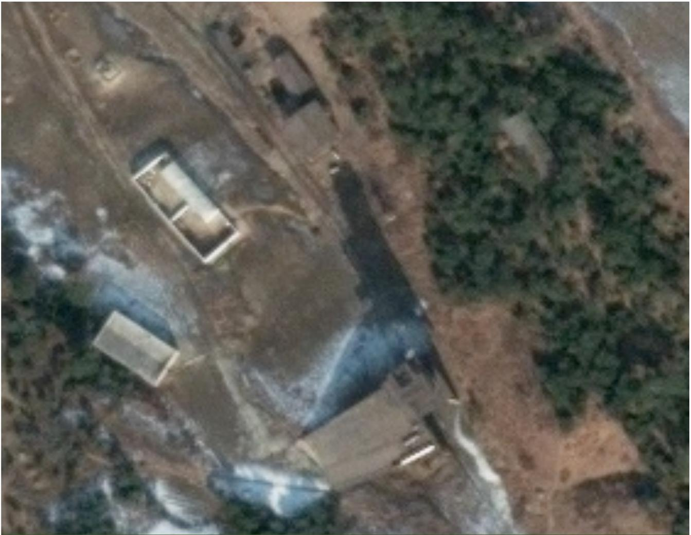
A close-up of the rocket engine test stand (bottom center) located approximately 500 m southwest of the main facility. The long shadow suggests that the tower has two, possibly three, platforms. The six buildings around the test stand are believed to be associated with it. The circular pad in the angle between the tower and closest support building is slightly obscured by snow and shadow (DigitalGlobe's Analysis Center).
