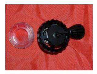
Malfunctioning OPV If the male threaded part attached to your lift bag or SMB is black in color then it is good and is <u>not</u> affected!
