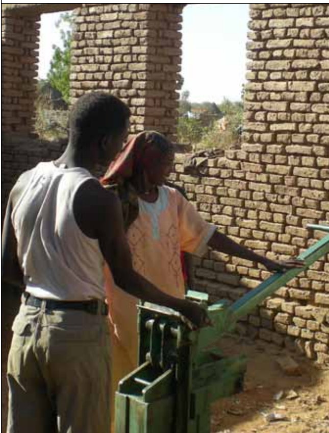
CRS is piloting a new construction technology that uses a block pressing machine to let schools make bricks out of soil, water and a bit of cement to build schools in West Darfur. Photo: CRS Staff.
