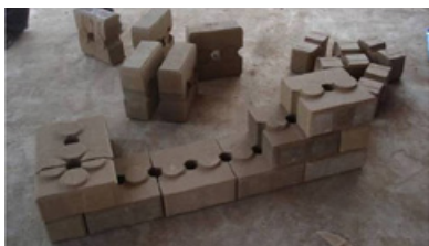
Compressed earth stabilised blocks (CSEB) were used as a sustainable and cheap construction material in some of the projects. Photo credit: CRS/Mehul Savla
