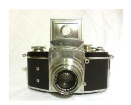
revolutionary camera. Besides being the first 35mm SLR (not the first SLR), it had interchangeable lenses, a focusing hood and magnifier, multiple shutter speeds from 12–1/1000 sec, a self timer, flash synch, even a built-in film cutter, and lots of other stuff. It was, and is, a great camera as well as a milestone product in the history of photographic technology.
