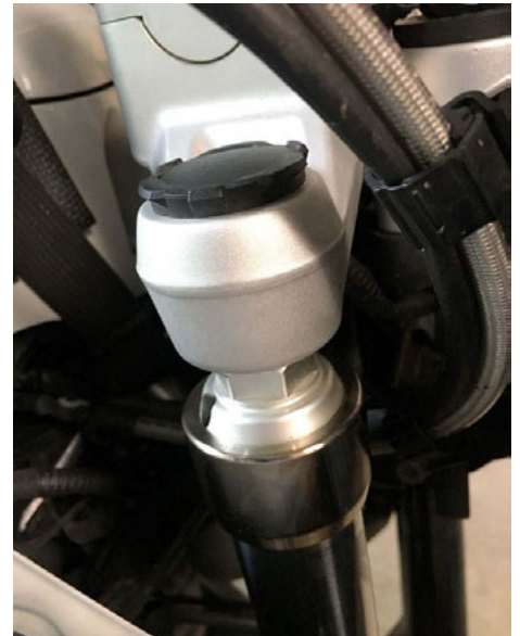
This photo, courtesy of Bob Aldridge, shows the collar BMW is attaching to the forks to prevent separation and possible failure.
