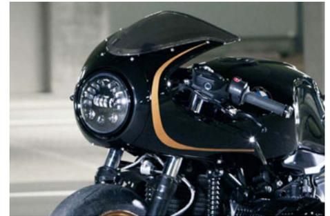
inserts. The bike retains the factory speedometer. The only thing we did there was weld a little bracket holder to the fairing so it sits within the fairing instead of on the yoke. The yoke was machined to remove the standard handlebar mounting points."
