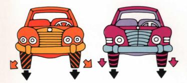
In the above left illustration you can see that the tire cord is wound on a bias which creates a force on the tire that does not run in the direction of the car's travel. The cord on the radial tire illustrated right is wound perpendicular to the line of travel. This eliminates the counter force, called rolling resistance, thereby, increasing gasoline mileage.
